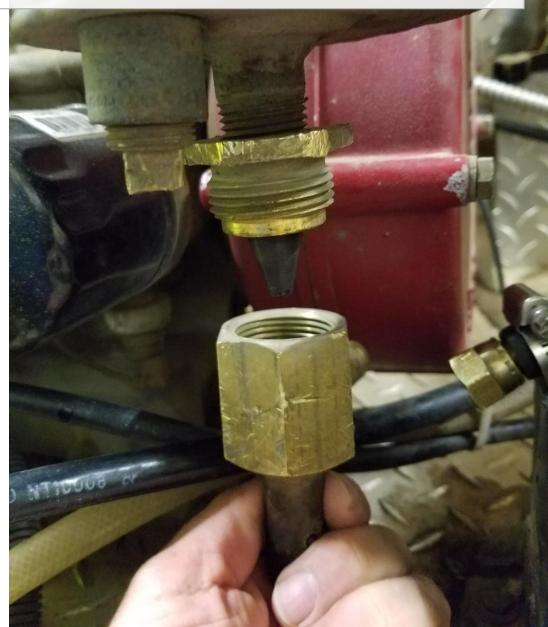
4. Remove debris from inside bottom of venturi until it's clean down to bare metal. This material is often soft enough to be wiped out, but scrape if necessary. The goal is to leave the funnel smooth.
