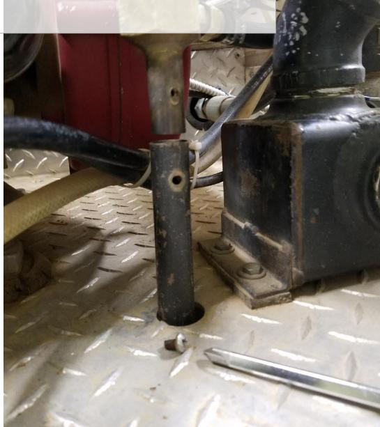
2. Remove vacuum line to pump discharge.
