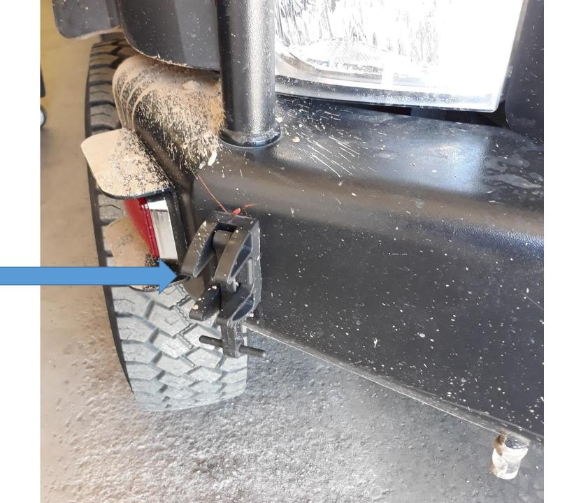
5531 also has the capability to spray water/foam while being driven over the fireline.
