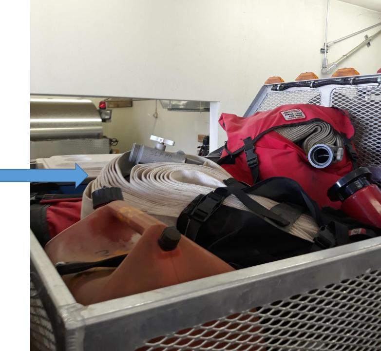
Top cover access to engine/pump compartment. Must be kept clear for air circulation to pump engine.
