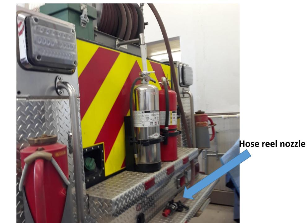
To prevent running over the hose when doing "Pump and Roll" bring the hose reel hose around and clip into clip on front bumper
