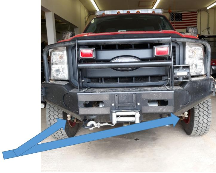
There are two spray heads under the front bumper Panel/Bumper outlet is set up for water or foam by pulling the lever and rotating the air control to obtain desired output.
