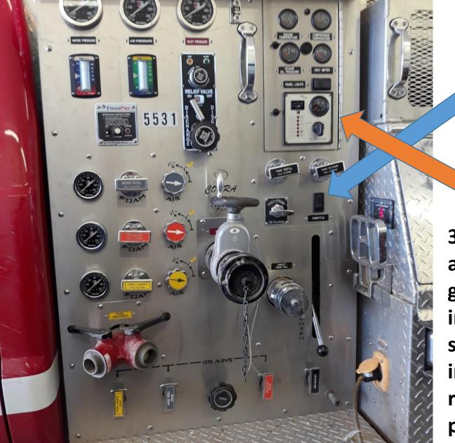
1. To start pump engine, open the throttle part way.
