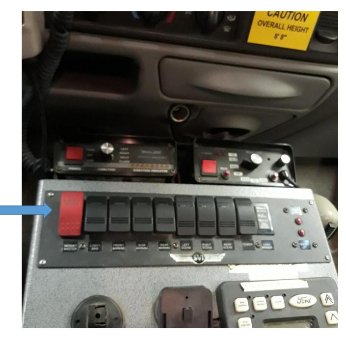
Charge Protect is used to hold the engine and the truck alternator at high idle to provide adequate current to maintain battery voltage
