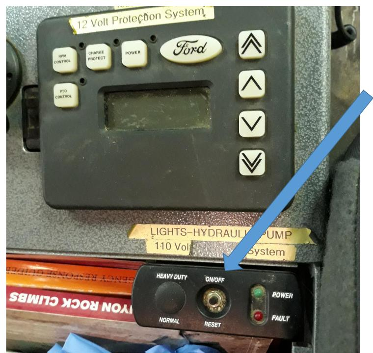
If there is need for 120/240 volt power, such as the overhead light tower, turn on the AC Alternator by depressing the ON/OFF Button.
