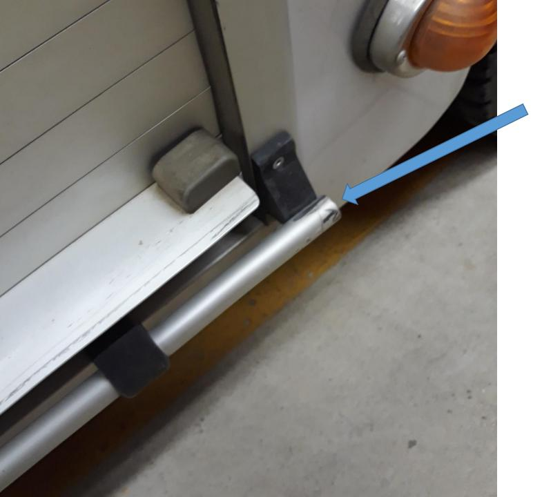
Latch not closed properly It needs to be pushed all the way against the black latch
