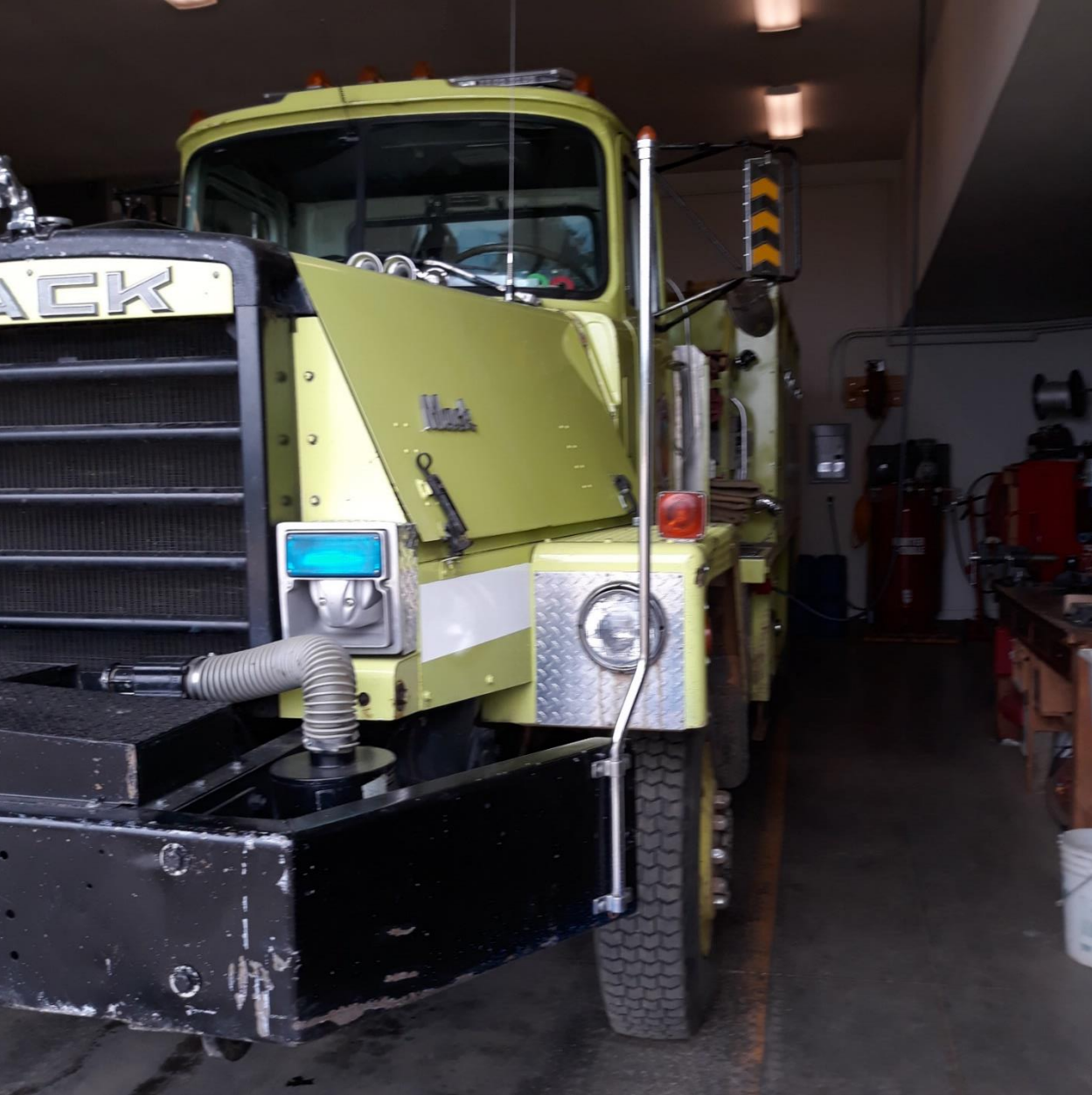
Front Mounted Air Compressor Electro-Magnetic clutch engages air compressor to front of engine crankshaft
